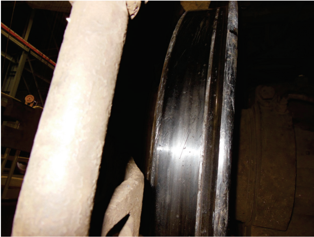
Locomotive 205 lead right hand wheel groove mark
