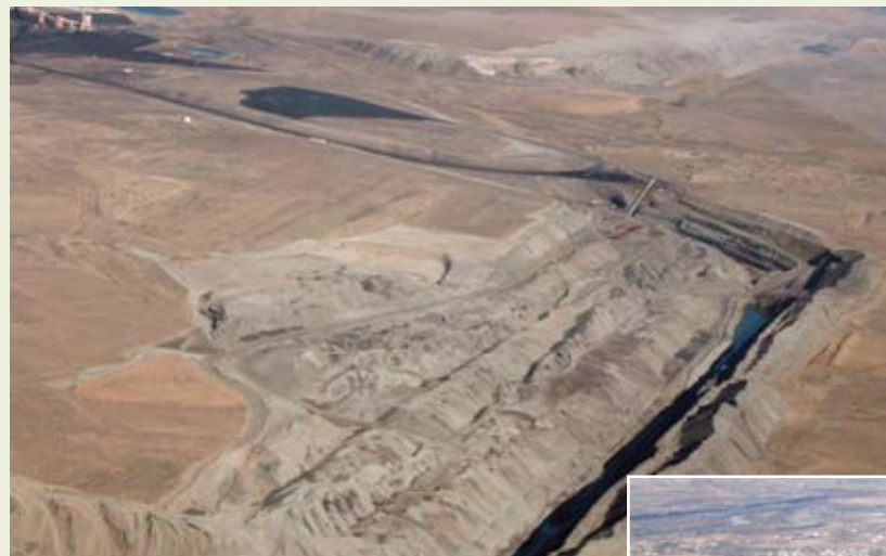
The 1,798-MW San Juan Generating Station generates about 1 million tons of CCW each year. A large quantity of the CCW is disposed in the San Juan Coal Mine.
