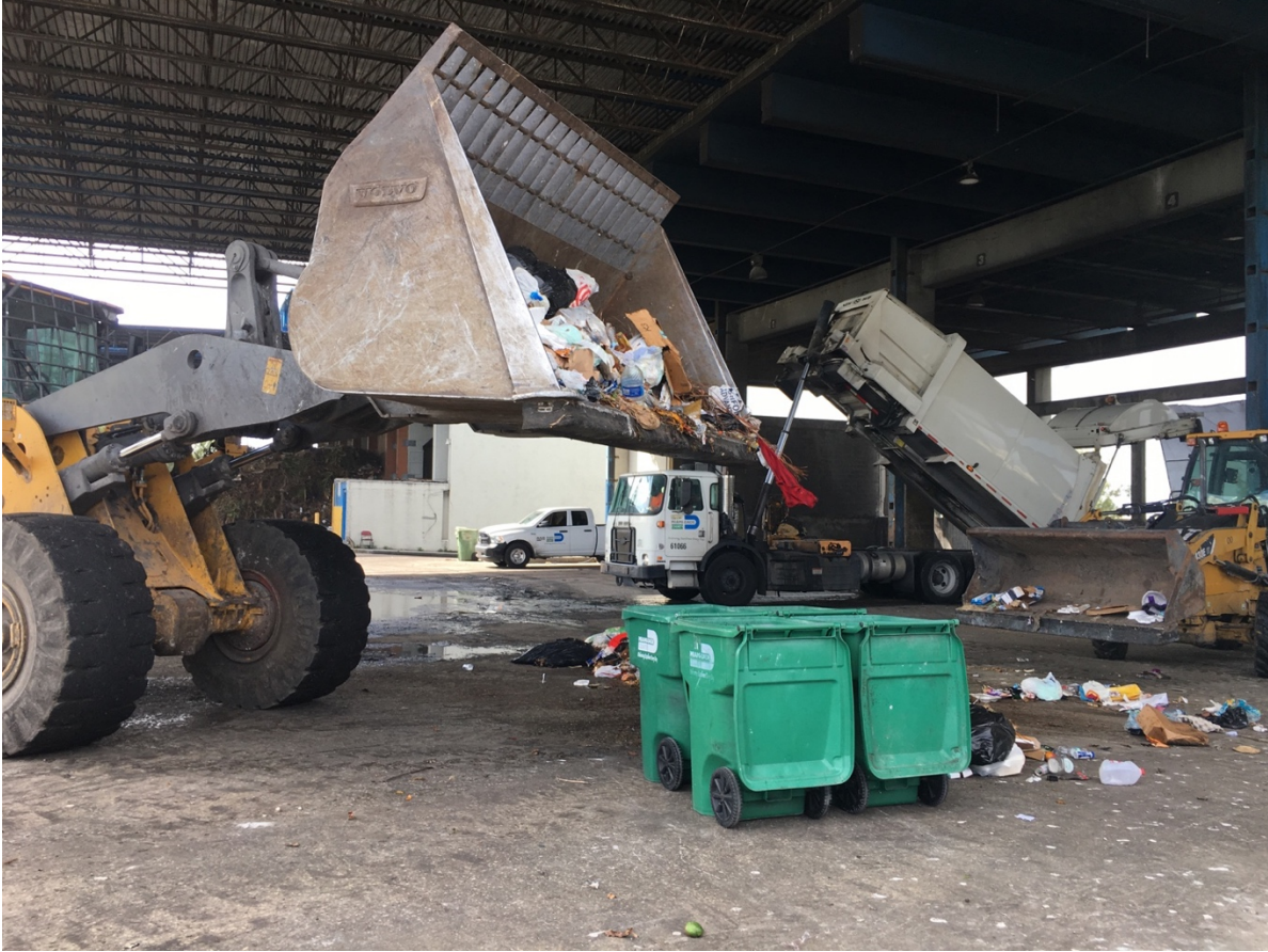
Figure 3. Front loaders dump a sample into roll carts at Northeast Transfer Station.
