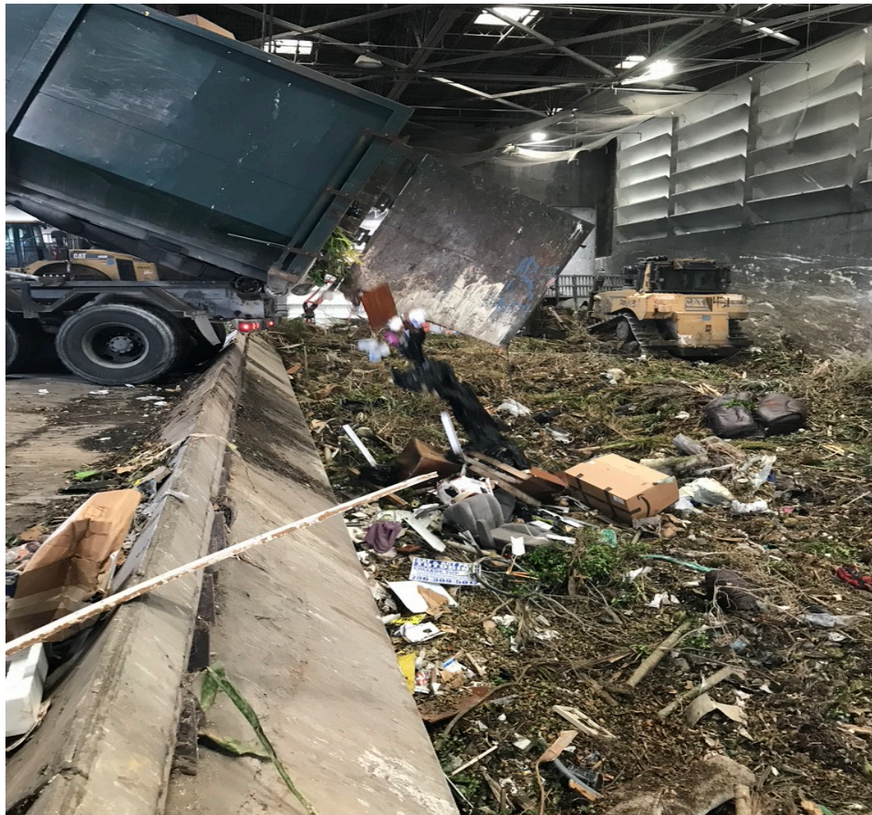
Figure 6. County trash truck dumps waste into the West Transfer Station surge pit.
