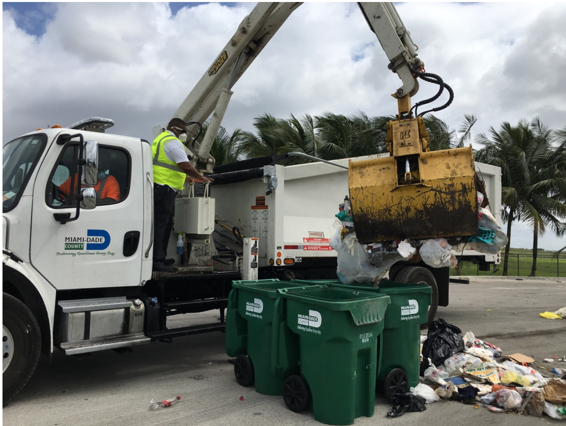
Figure 2. A truck-mounted clamshell bucket loads a sample into roll carts at Resource Recovery.
