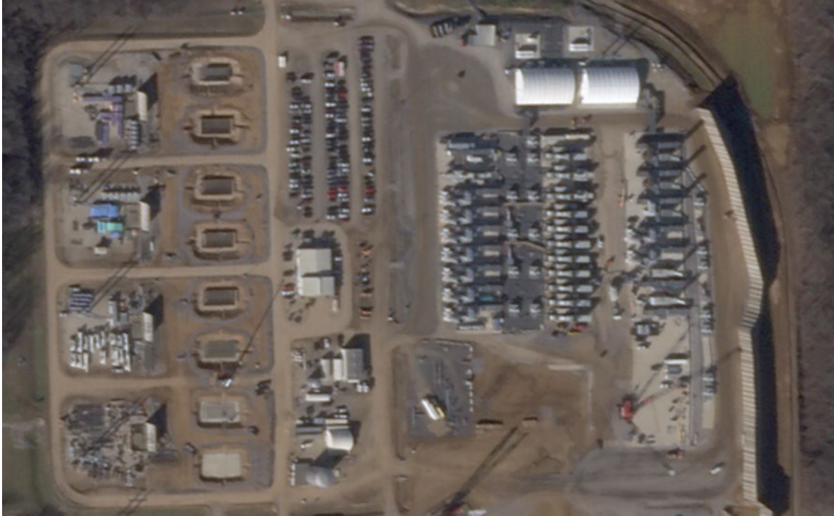
Figure 4: Close-up aerial image of xAI's Stanton Road S. facility showing 27 turbines (Feb. 9, 2026).
