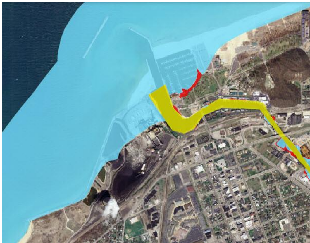
Figure 4. 100-year floodplain at the NIPSCO Michigan City Generating Station obtained from FEMA Flood Rate Insurance Maps, accessed at maps.Indiana.edu .
