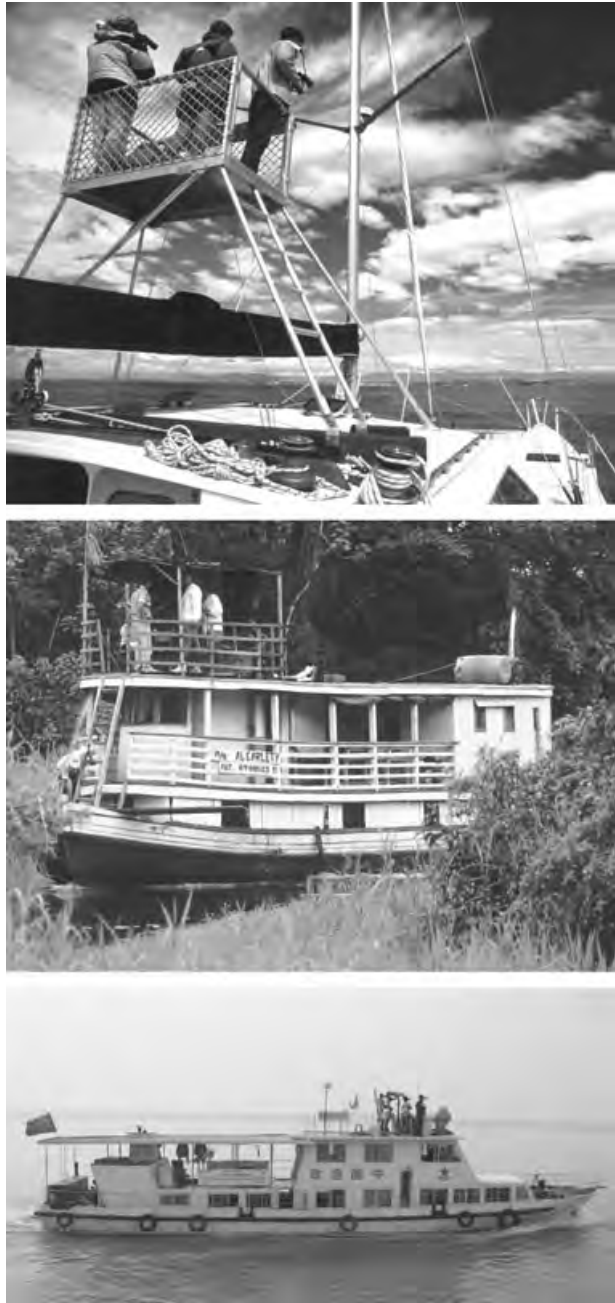
Fig. 1. Examples of small vessels used in coastal and riverine line-transect surveys. Note the raised sighting platforms, which give eye heights between 4.5 and 6 m.
