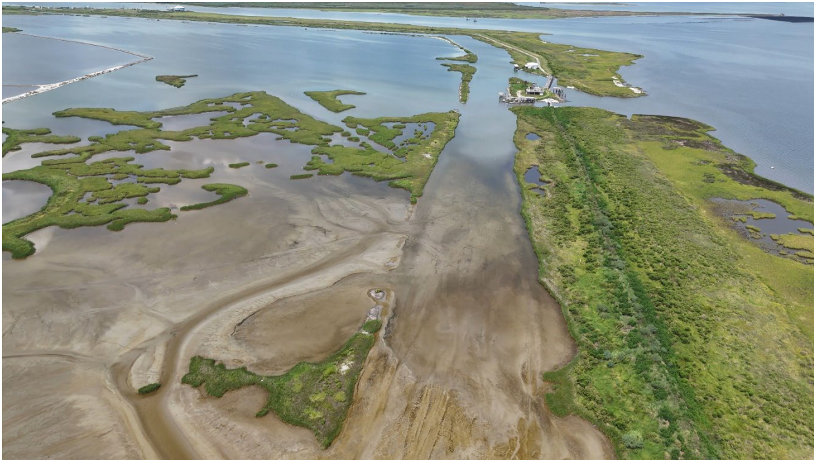
Figure 4, looking West, dredged material filling No Name Bayou near the No Name Weir. The weir can be seen in the upper left corner of the image.
