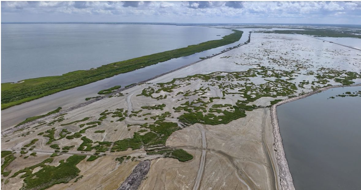
Figure 2 , looking ENE, discharged dredged material in the Refuge; No Name Bayou (near the No Name Weir) can be seen partially filled alongside vegetated barrier between the bayou and Calcasieu Lake (lower left side).
