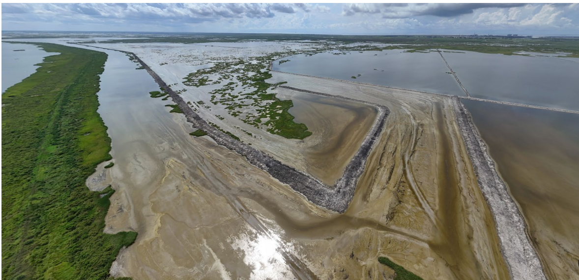
Figure 3 , looking ESE, dredged material discharges in and partial fill of No Name Bayou (lower side) near the No Name Weir; Calcasieu Lake visible in upper left quadrant.
