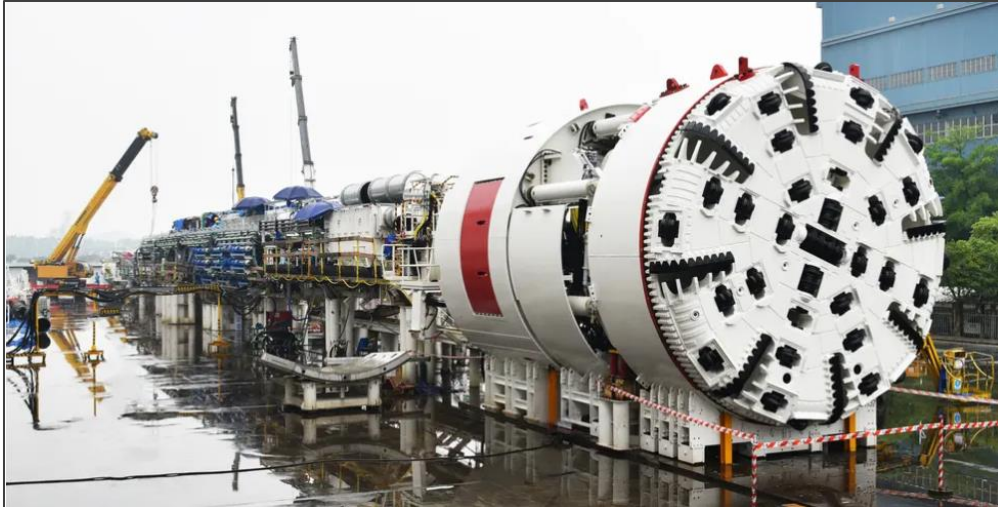
Figure 2. A tunnel boring machine similar to the one planned for use in the L5TP. The machine consists of a rotating cutting head and "trailing gear" that extends several hundred feet behind the cutting head (580 feet for the L5TP TBM). The example shown was used for subway tunnel construction in Sydney, Australia ( https://www.sydneymetro.info/article/first-mega-borer-its-way-city-tunnelling ).
