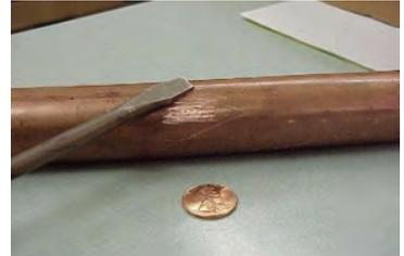
When performing a scratch test, if it turns shiny silver, like the image above, it is likely lead. If the scratched area turns yellow-orange, it is likely copper.
