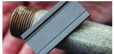
Galvanized iron pipe can also be silver in color, to distinguish between lead and galvanized iron, place a magnet on the pipe. If the magnet sticks to the pipe, it's likely iron and not lead.
