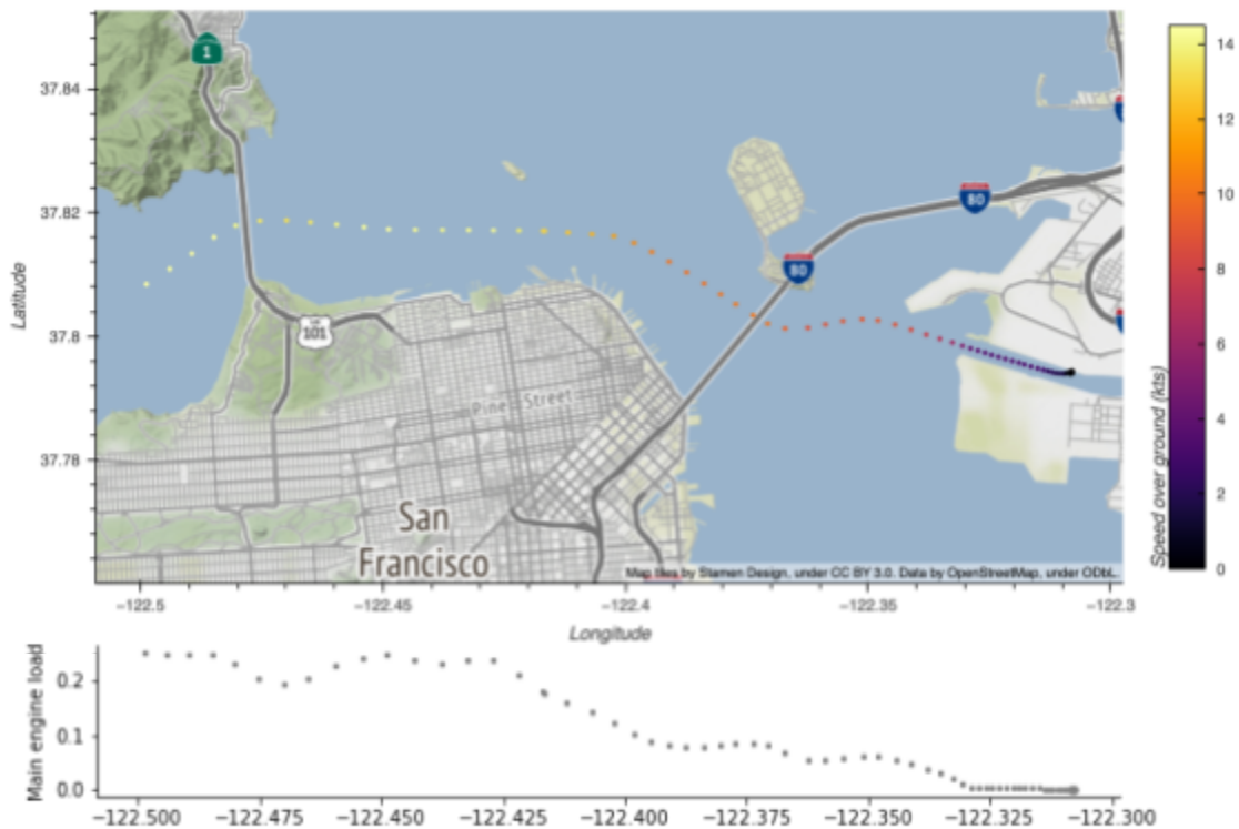
Figure 3: Speed over ground, positions, and main engine load for the inbound leg of the MSC Amsterdam calling at the Port of Oakland
