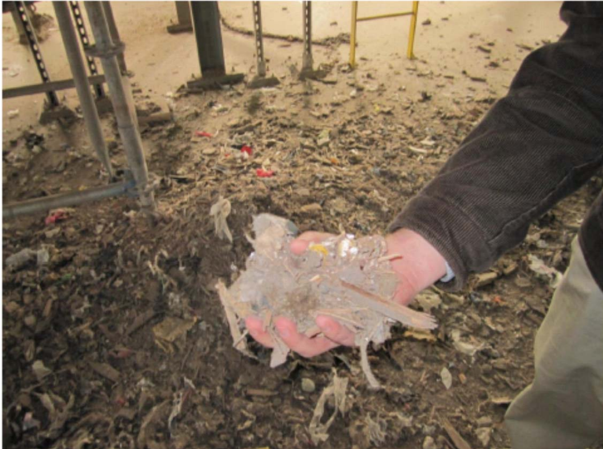
Fig.1: Boiler fuel made from “forest industry waste, shredded construction wood waste, and demolition debris.” 6
