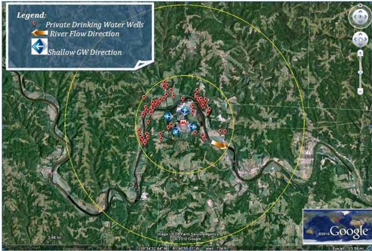
Mounding of groundwater in the disposal area may cause localized flow in other directions.
