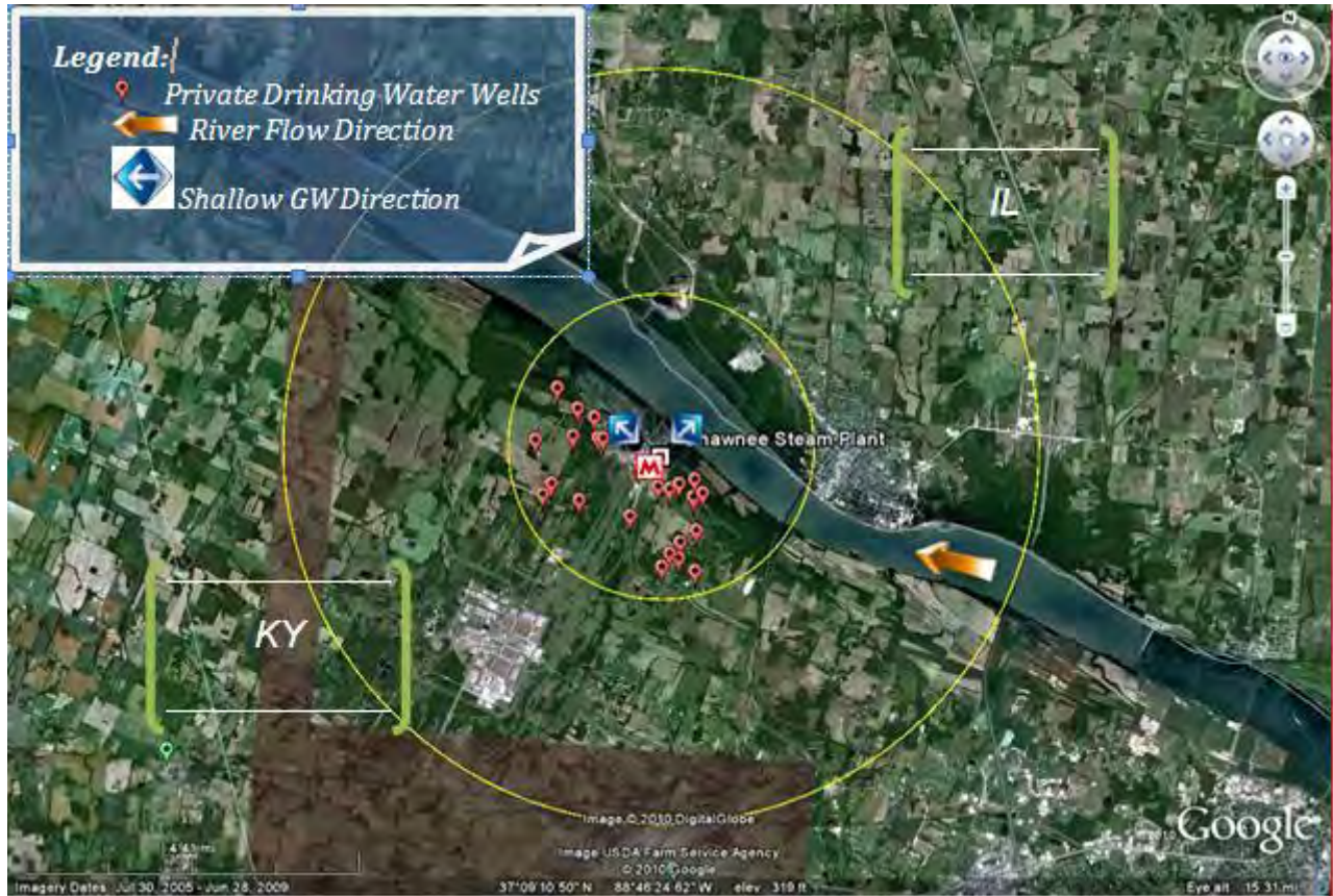
Mounding of groundwater in the disposal area causes localized flow in all directions.
