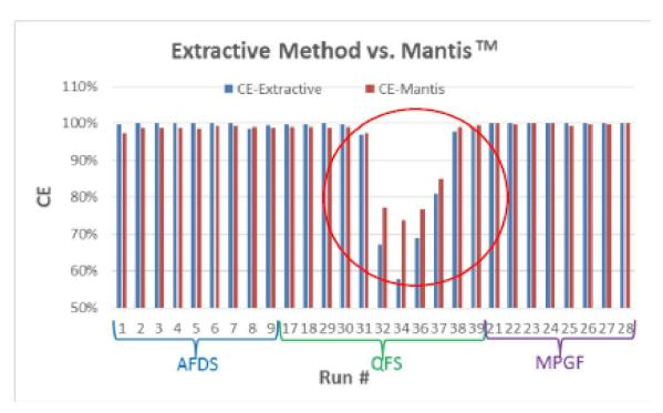
As the chart shows, even under controlled conditions a flare's control efficiency ("CE"), and by extension destruction efficiency, can drop to very low values (55% or so in this case). So, the Division's simple assumption that destruction efficiencies will be 98%, Proposed Permit § II, Cond. 8.1, is not realistic and the evidence establishes that achieving such rates is not consistently achievable, such as with rapidly varying flow rates and waste gas compositions.
