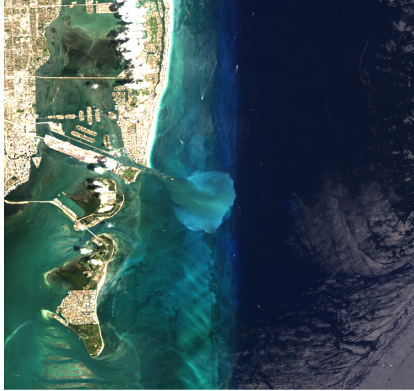
Figure 3. Landsat image accessed April 24, 2014 showing an immense plume of turbidity at the Port of Miami.
