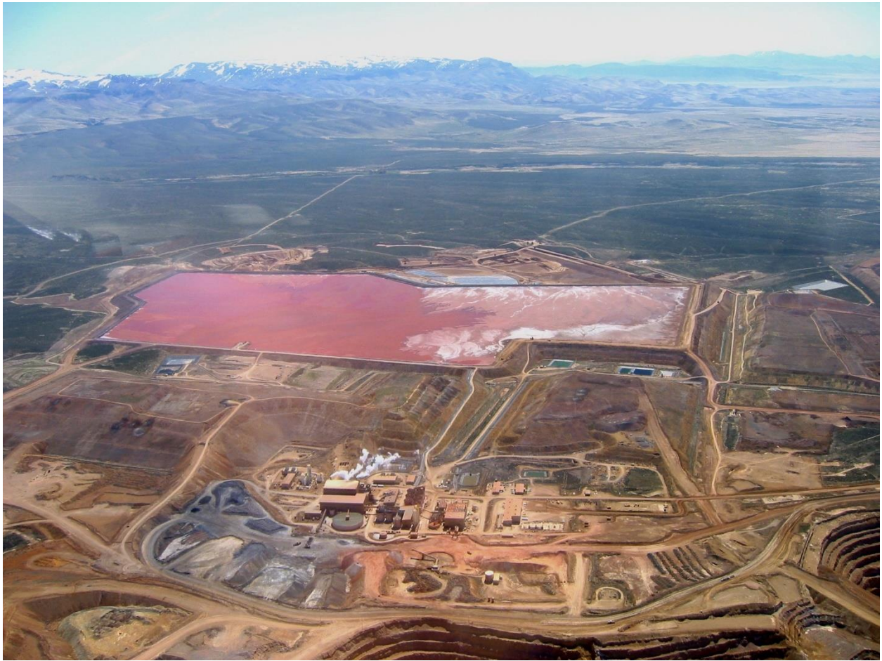
The Twin Creeks Mine, Humboldt County, Nevada. This mine uses cyanide leaching to extract gold. The red object in the photo is the surface of the tailings pond water, which is not covered. The edge of one of the mine pits appears in the bottom right side of the photo. Since this photo was taken, the tailings pond has been expanded backward from the facility shown.
