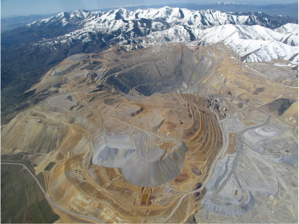
The Bingham Canyon Mine, AKA the Kennecott Copper Mine, Salt Lake County, Utah. This open pit copper mine's pit is more than half a mile deep and covers 1,900 acres.
