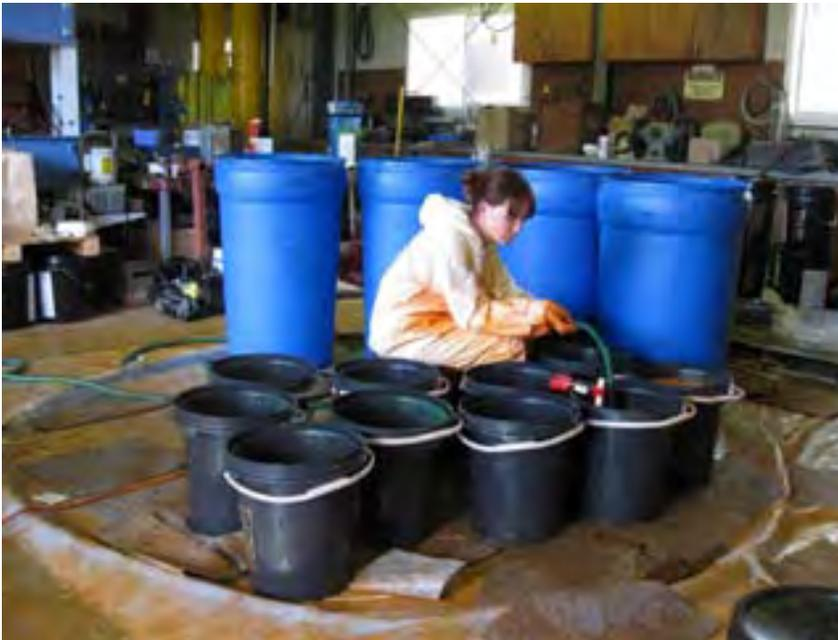
Figure 4-6: Transferring fluorescein concentrate to 5 gal. buckets for delivery to wells.
