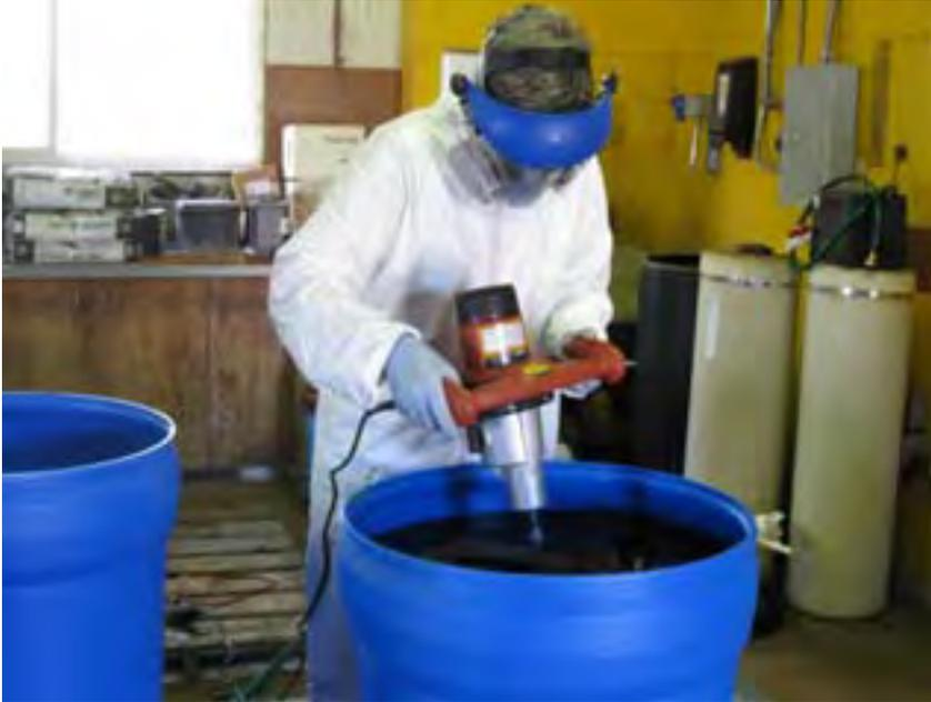
Figure 4-5: Mixing fluorescein in 55 gal. drums.
