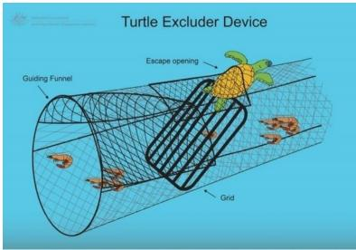
Figure 3. TED diagram. Source: NMFS, Environmental Impact Statement to Reduce the Incidental Bycatch and Mortality of Sea Turtles in the Southeastern U.S. Shrimp Fisheries (Final) at vi (2019) [hereinafter FEIS].
