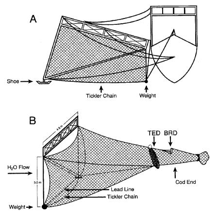
Figure 2. Diagram of typical skimmer trawl with a TED installed. The "BRD" is a bycatch reduction device used to allow finfish to escape from the trawl. Source: NMFS, Reinitiation of Endangered Species Act (ESA) Section 7 Consultation on the Continued Implementation of the Sea Turtle Conservation Regulations under the ESA and the Continued Authorization of the Southeast U.S. Shrimp Fisheries in Federal Waters under the Magnuson-Stevens Fishery Management and Conservation Act (MSFMCA) 22 (2014).
