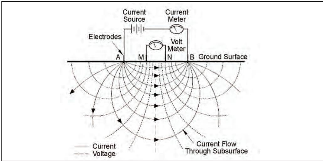
ERI techniques can be applied either over-land with an array of electrodes spaced along the survey boundary or along the sea bed using a towed sled with a multi-electrode “streamer” cable attached. Typically, the deeper the penetration desired, the longer the electrode array or streamer cable will need to be. Penetration depths are generally on the order of about 15 feet. Greater depths are possible, but at the expense of decreased accuracy and resolution.
