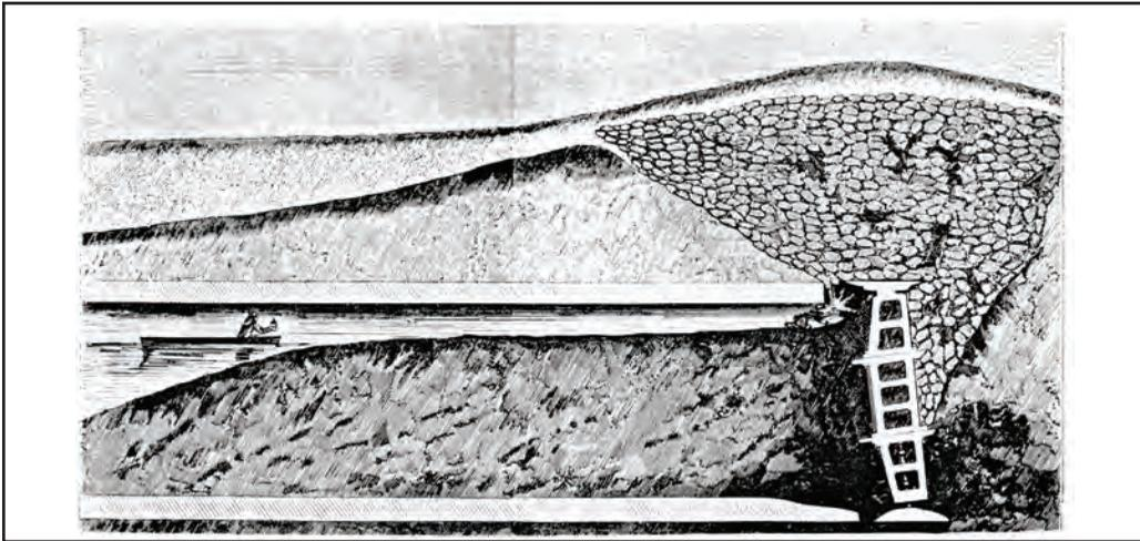
(Sketch indicates Brunel's shield, at right, after a breach and flooding. The shield has been "buried" with a soil plug above in an attempt to seal the leak so that the tunnel can be pumped dry and excavation can resume.)
