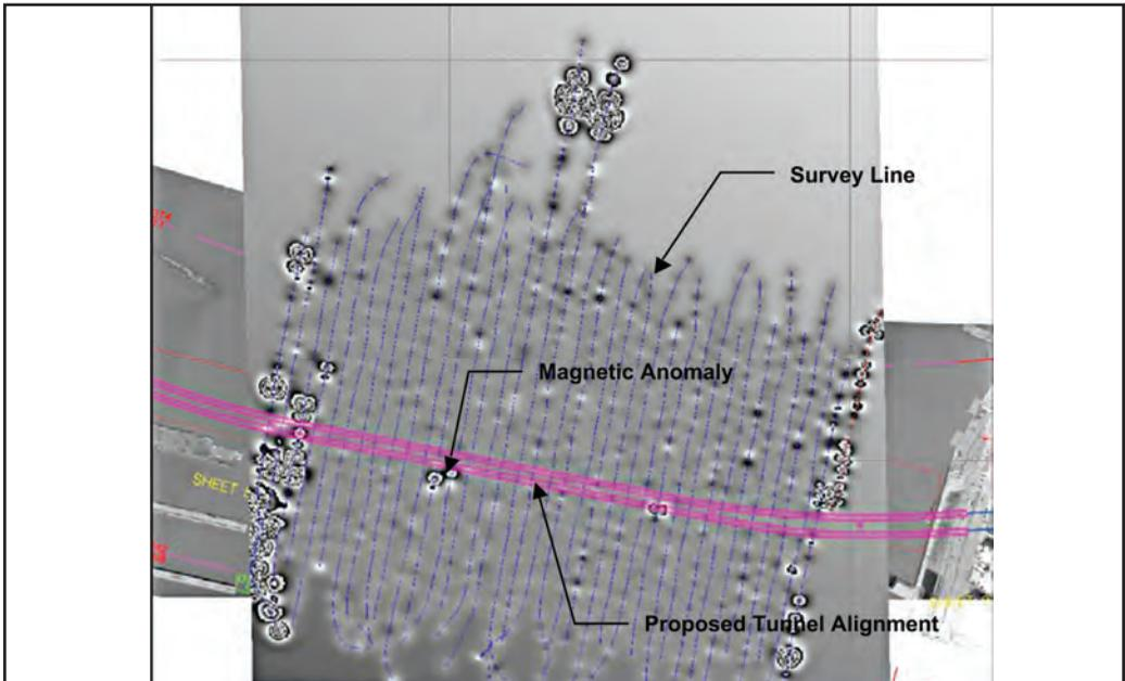
Gradiometer surveys use the same principles of magnetometer surveys but can utilize multiple magnetic instruments coupled with powerful software to locate magnetic anomalies by triangulation. Gradiometer instruments are capable of filtering background “noise” such as diurnal effects and influences from surface debris. Several types of gradiometer instruments are available and their application varies depending on the type of anomaly being investigated as well as other environmental factors.
