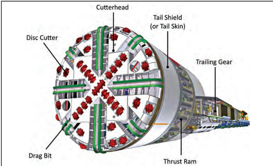
TBMs perform the following functional activities: boring (or cutting), thrusting, mucking, and installation of ground support (the tunnel lining), all within the enclosure of the machine. Steering and alignment control is contained within the machine and adjustments to the tunnel alignment can be made with gripper “shoes” or jacks mounted on the main support beam of the TBM or by adjusting the force applied at the thrust rams against the installed tunnel lining.
