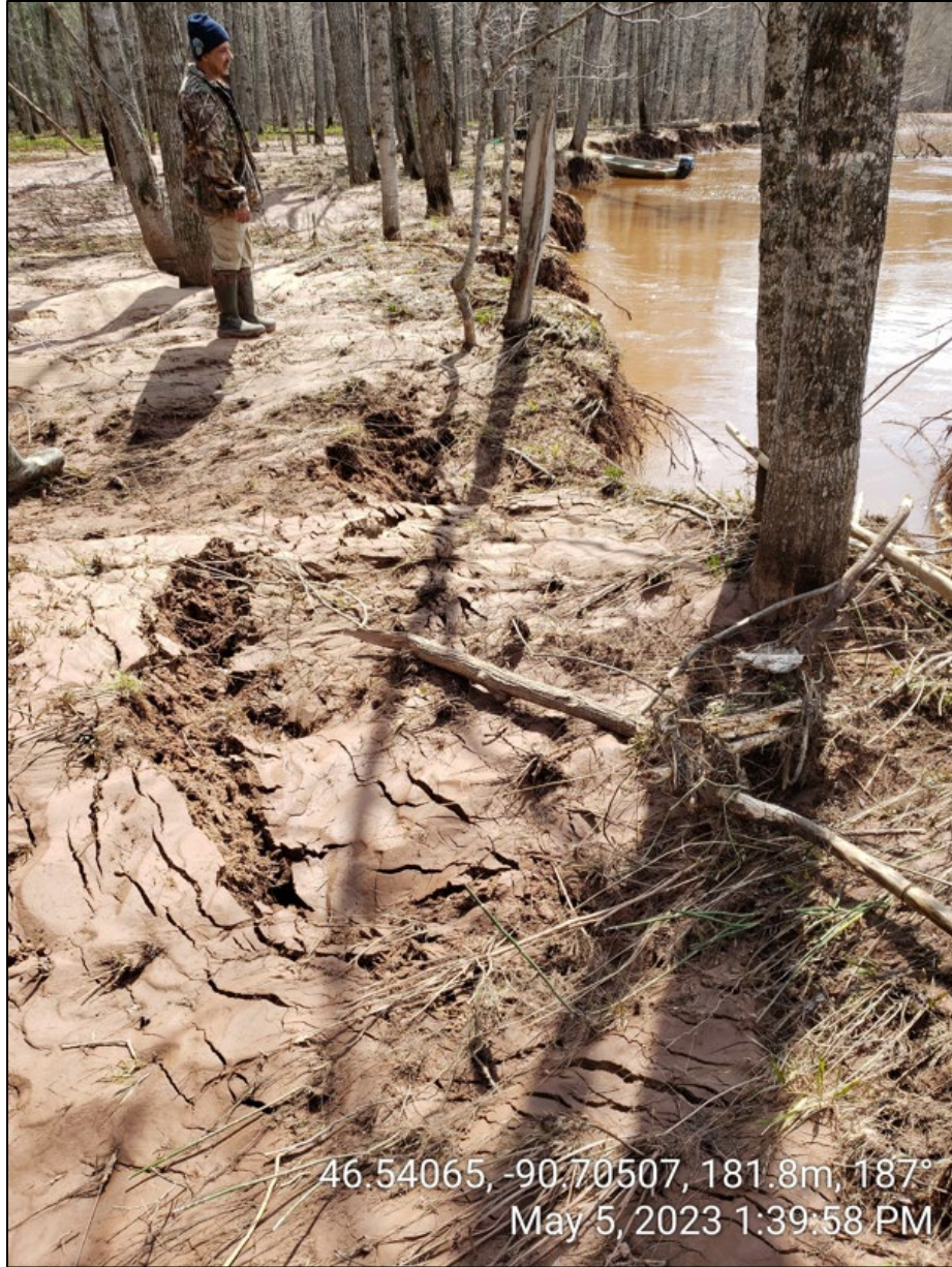
Figure 6. Photograph of cracks in channel bank at upstream end of meander neck taken on May 5, 2023.
