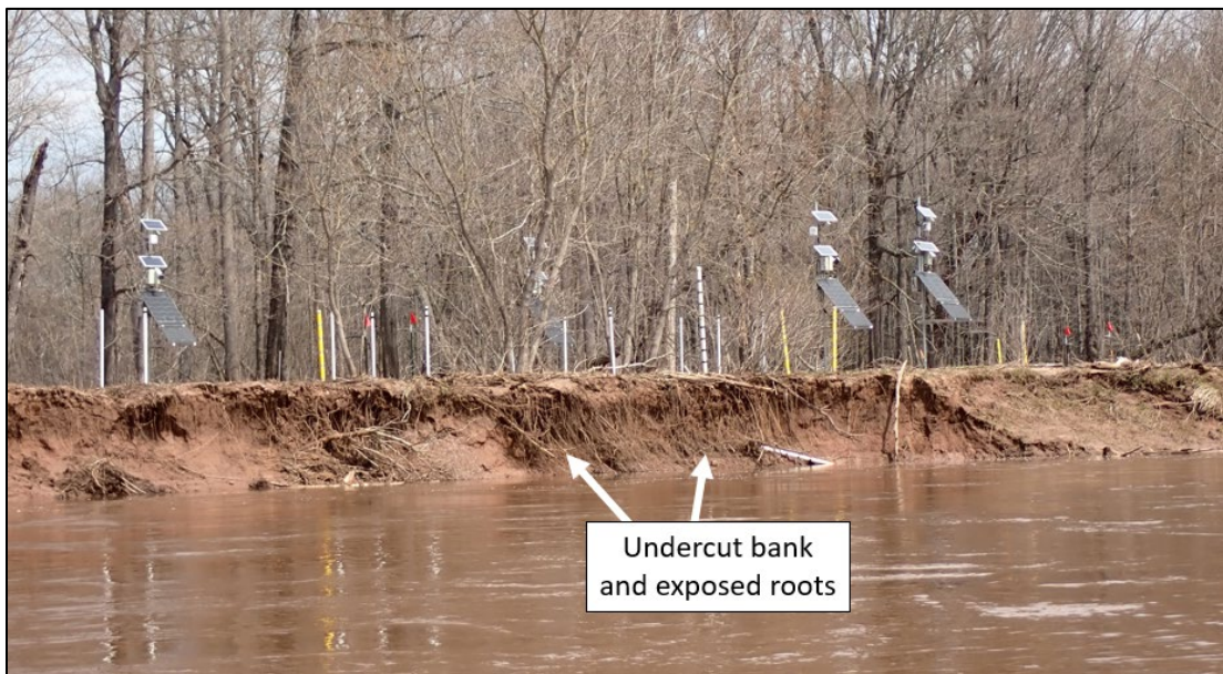
Figure 8. Photo from May 8 showing undercut bank and overhanging roots.
