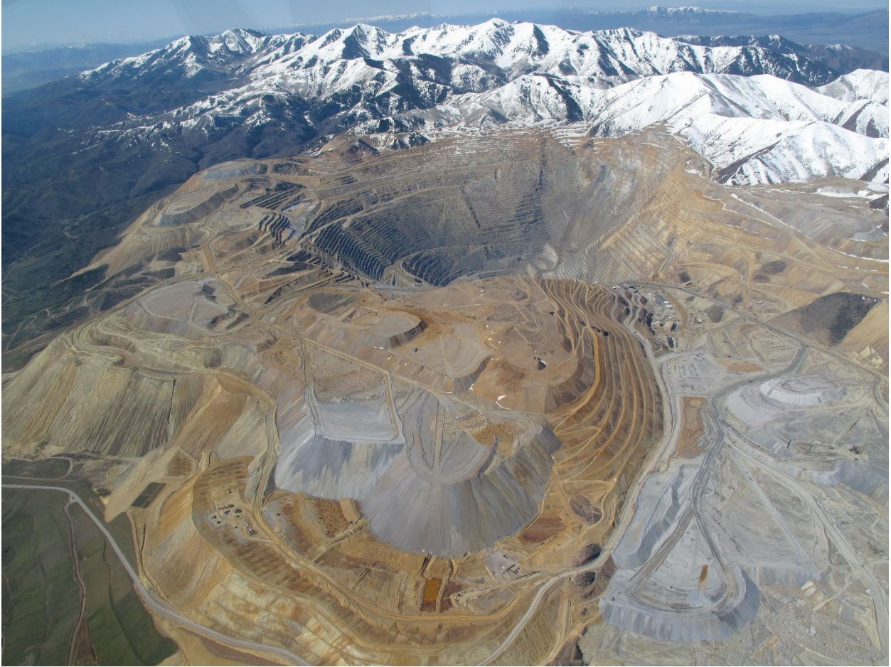
The Bingham Canyon Mine, aka the Kennecott Copper Mine, Salt Lake County, Utah. This open pit copper mine's pit is more than half a mile deep and covers 1,900 acres. Groundwater pollution from the mine extends over tens of square miles.
