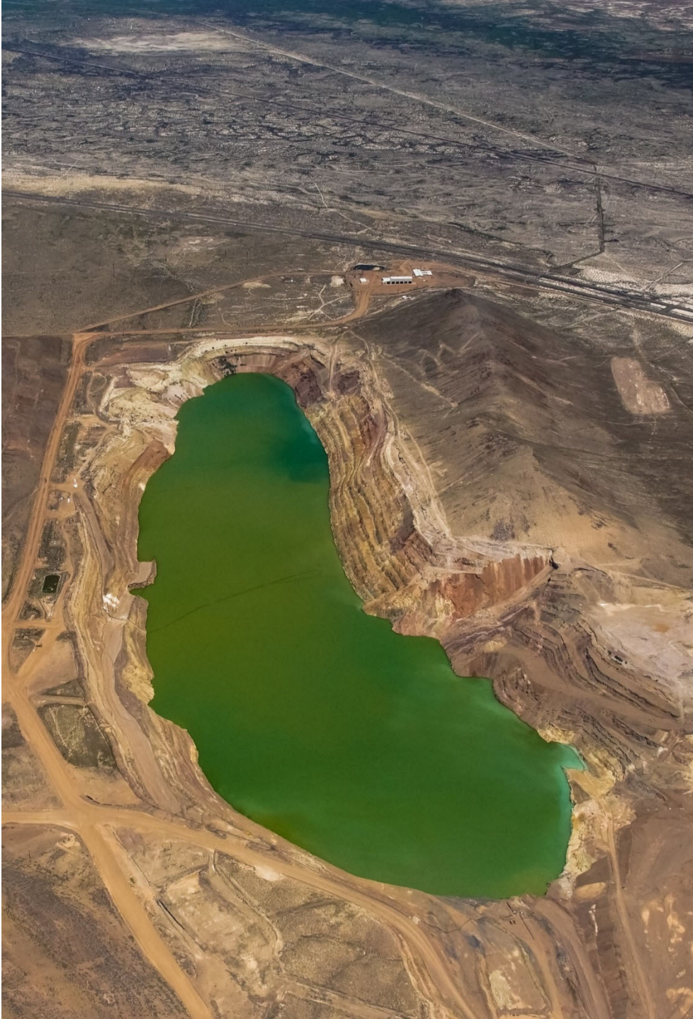
The Lone Tree Mine, Humboldt County, Nevada. This mine used cyanide leaching to extract gold and silver. Mining finished in 2007. The water body in the photo is the former mine pit, now a contaminated “lake” that requires long-term management.
