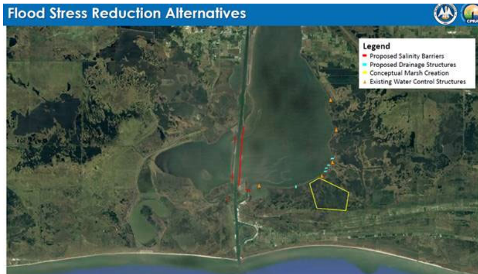
Figure 5. Flood stress reduction and salinity control measures along the CSC and Calcasieu Lake rim as proposed by CPRA. 165
